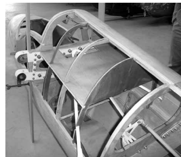
Forward fuselage, controls and wing supports with the elevator pushrod Photo: John McCorquodale
