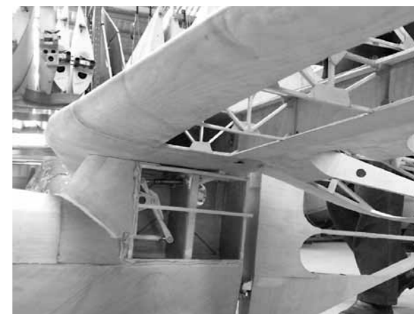
Tail group, the rudder is easily removed to allow the tailplane to be fitted or removed Photo: Cliff Pritchard
