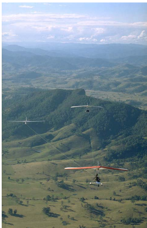
A "trike" showing it's versatility towing a hang glider and a sailplane
