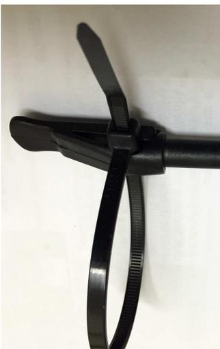
If you are unable to test your latches for security a cable tie can be tensioned around the latch when the latch is closed.
