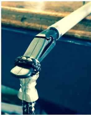
The latch fittings are batch tested prior to production to ensure conformity to the design requirements. To check your hinge batten fitting. The wing should be de-tensioned and the battens should be removed from the sail. Secure batten to a bench.
